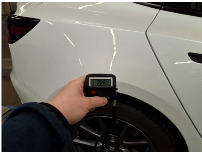
Repainting 1: Side panel - rear left side, Side panel - rear right side, Door - rear left side, Door - rear right side, Door - front right side
