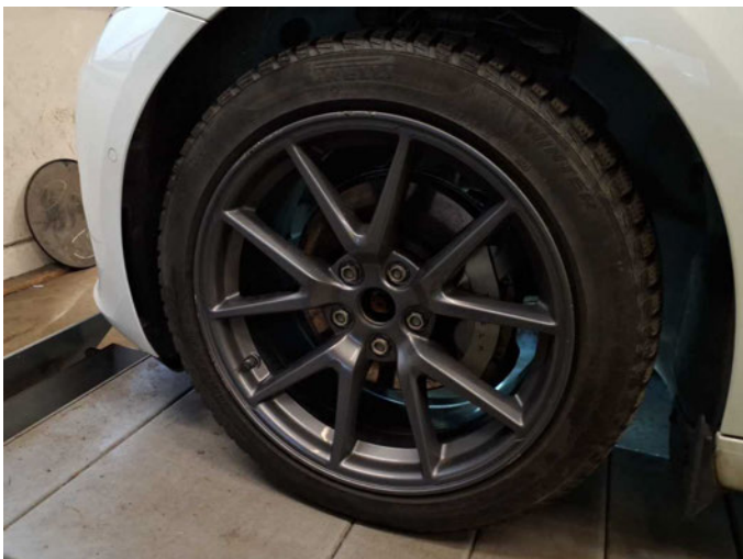
Damage 9: Wheel / tyres: Alloy rim - front left side - Scratched - Replace
