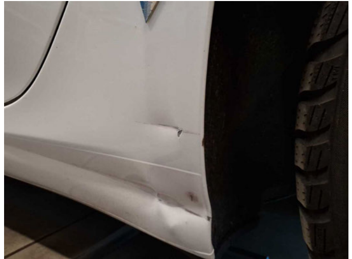
Damage 11: Sill - left side: Sill - Deformed - Repair and paint
