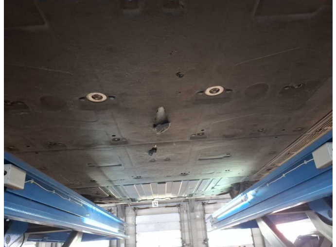
Damage 3: Body: Underbody panelling - Damaged - Replace
