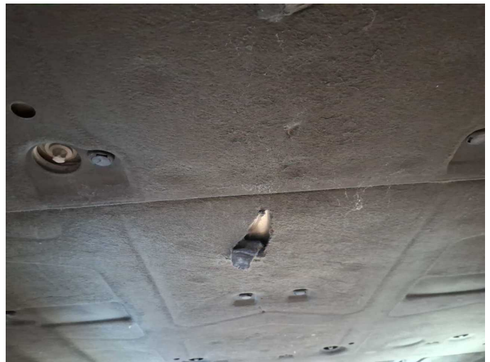
Damage 3: Body: Underbody panelling - Damaged - Replace
