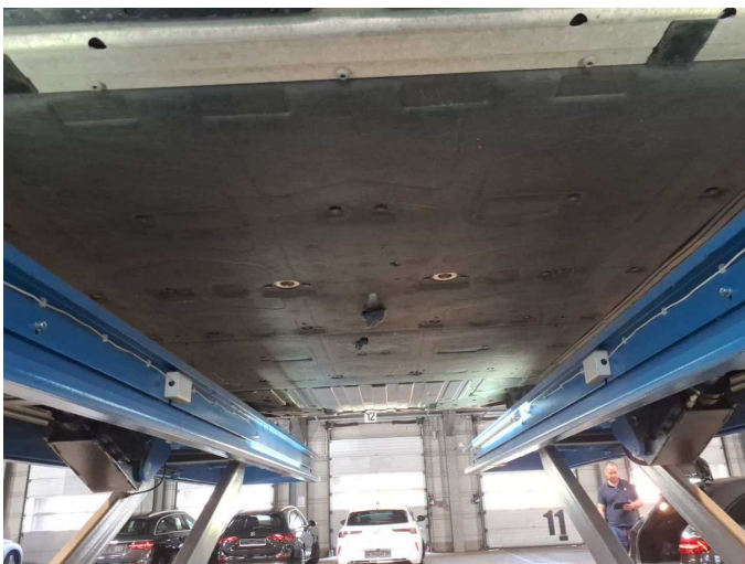
Damage 3: Body: Underbody panelling - Damaged - Replace
