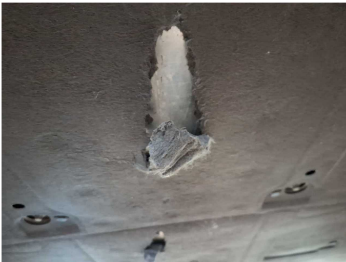
Damage 3: Body: Underbody panelling - Damaged - Replace
