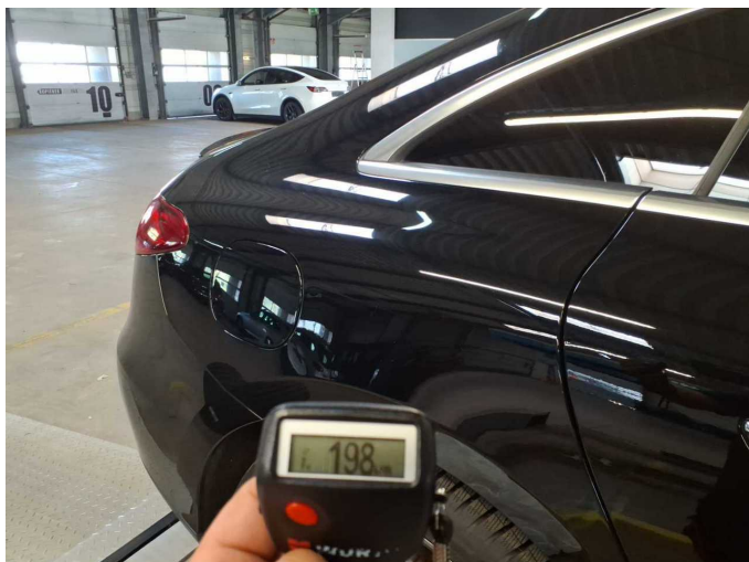
Repainting 1: Side panel - rear right side
