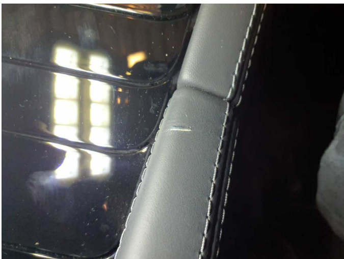
Damage 2: Instrument panel: Centre console - front - Scratch(es) - Smart repair
