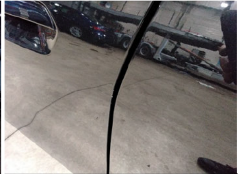
Tür / Vorne Links / Kratzer
