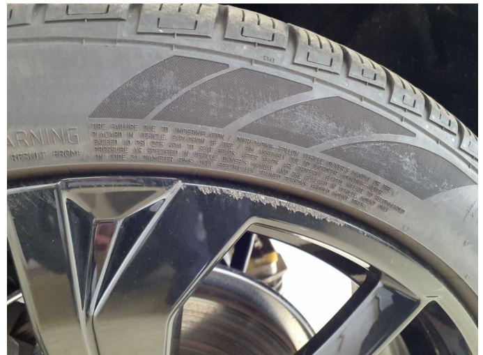
Damage 11: Wheel / tyres: Alloy rim - rear left side - Scratched - Loss in value
