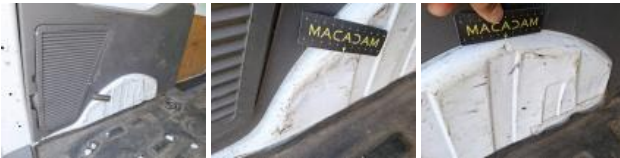
Wheel aperture RR, Dent(s) and scratch(es), Spot repair
