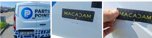
Bumper moulding R, Dent(s) and scratch(es), Repair and paint (complete)
