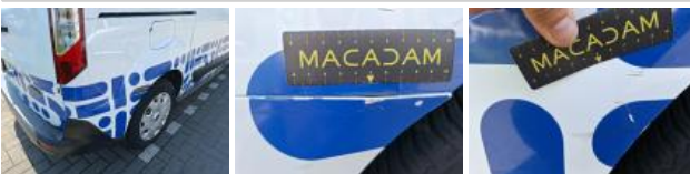
Bumper moulding R, Dent(s) and scratch(es), Repair and paint (complete)
