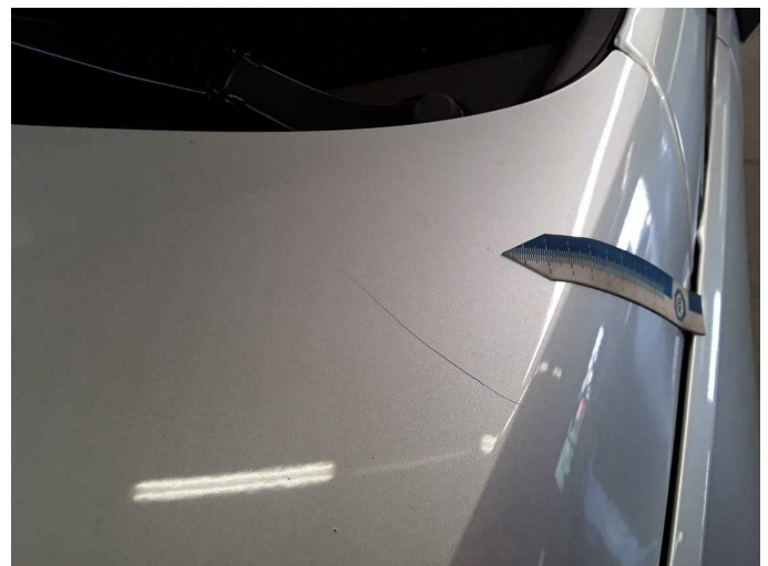
Damage 12: Bonnet: Bonnet - Dent / paintcoat damage - Paint
