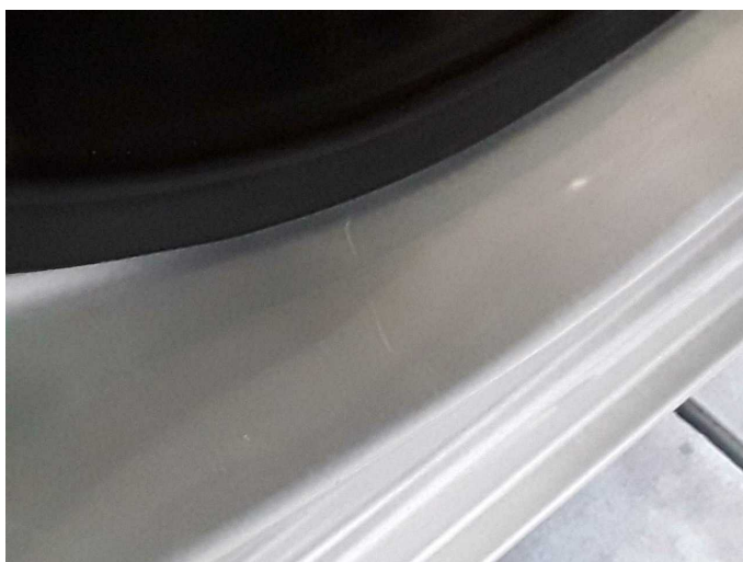
Wear and tear 3: Side panel - rear right side: Sill - Scratch(es) - No deduction
