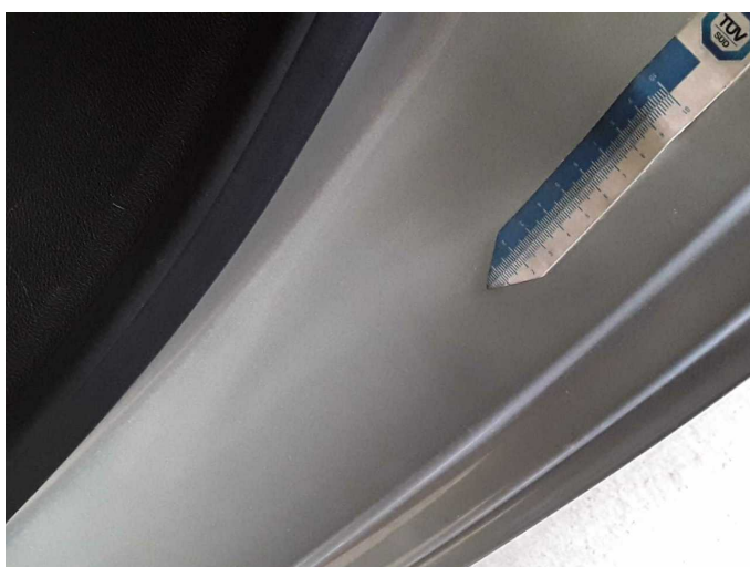
Wear and tear 1: Side panel - rear left side: Sill - Scratch(es) - No deduction
