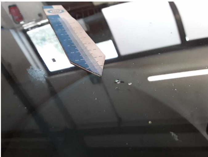
Damage 10: Vehicle glazing: Windscreen - Stone chips - Replace
