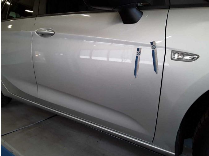
Damage 5: Door - front right side: Door - Scratched - Paint
