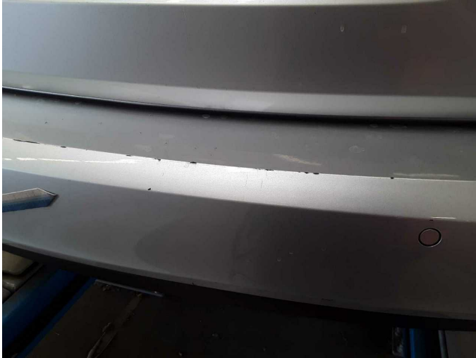
Damage 8: Rear bumper: Rear bumper - Scratched - Paint
