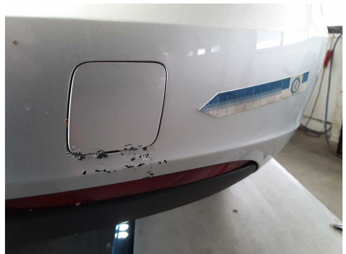
Damage 8: Rear bumper: Rear bumper - Scratched - Paint
