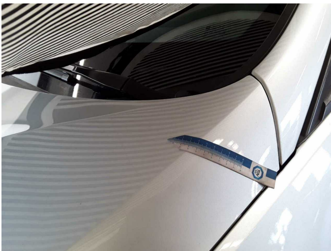
Damage 12: Bonnet: Bonnet - Dent / paintcoat damage - Paint
