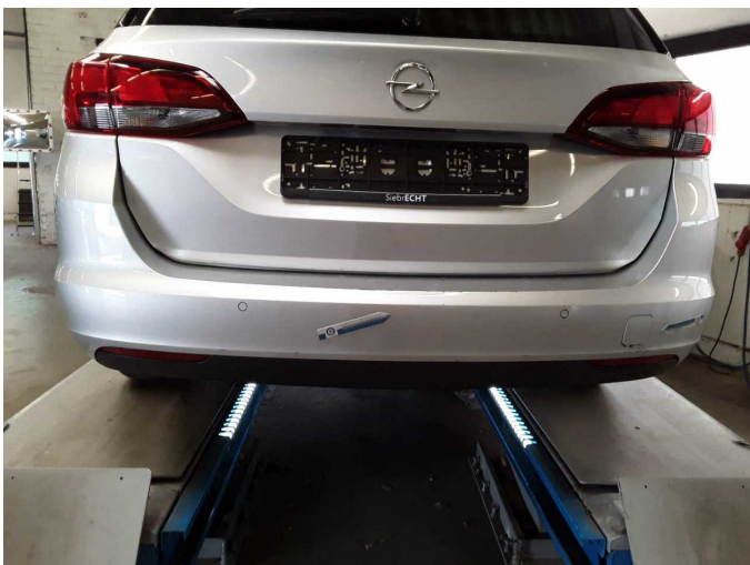
Damage 8: Rear bumper: Rear bumper - Scratched - Paint
