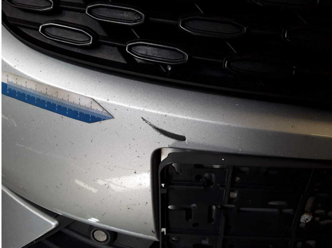
Damage 9: Front bumper: Front bumper - Scratched - Paint
