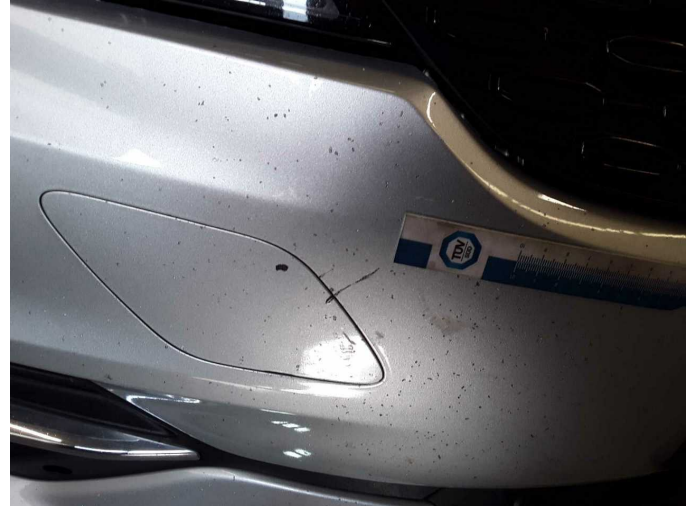
Damage 9: Front bumper: Front bumper - Scratched - Paint
