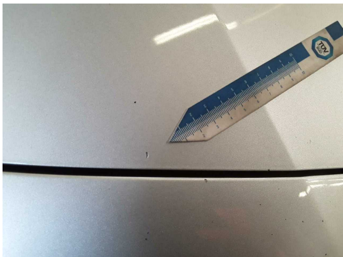
Damage 12: Bonnet: Bonnet - Dent / paintcoat damage - Paint
