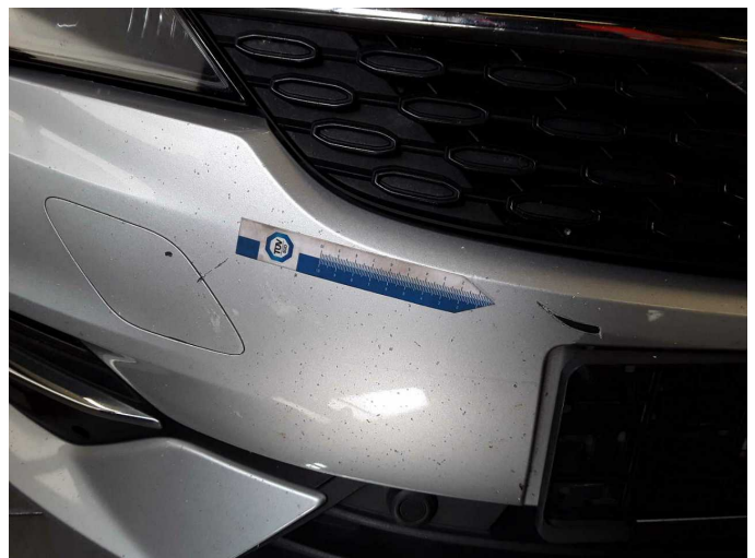
Damage 9: Front bumper: Front bumper - Scratched - Paint
