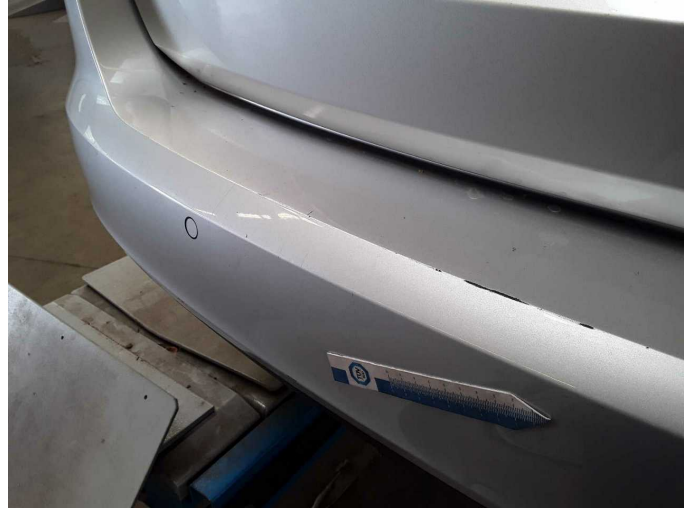
Damage 8: Rear bumper: Rear bumper - Scratched - Paint
