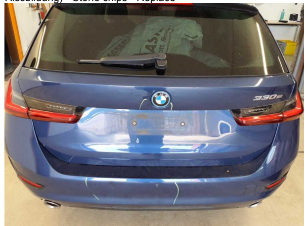
Damage #7: Boot lid / rear door: Boot lid - dent(s) - Repair and paint
