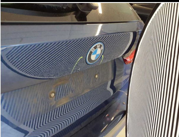
Damage #7: Boot lid / rear door: Boot lid - dent(s) - Repair and paint
