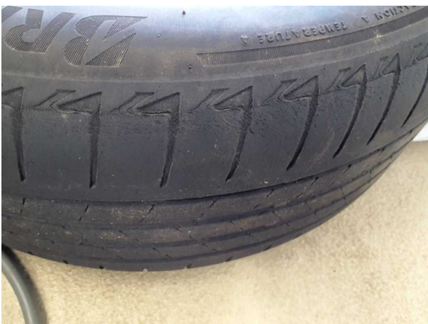
Damage #3: 2nd wheel set: 2 tyres - Worn - Replace
