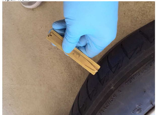
Damage #3: 2nd wheel set: 2 tyres - Worn - Replace
