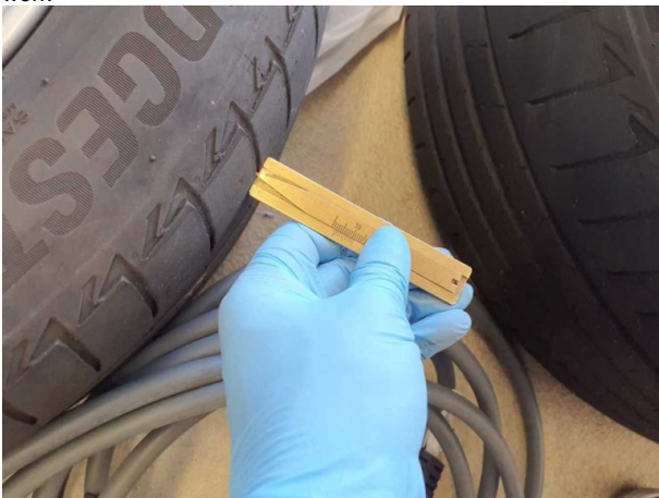
Damage #3: 2nd wheel set: 2 tyres - Worn - Replace
