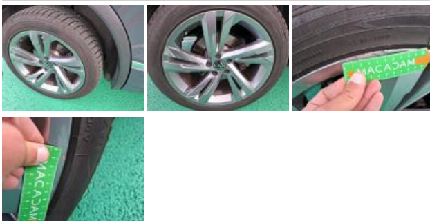
Tyre FR, Out of tolerance, Replace
