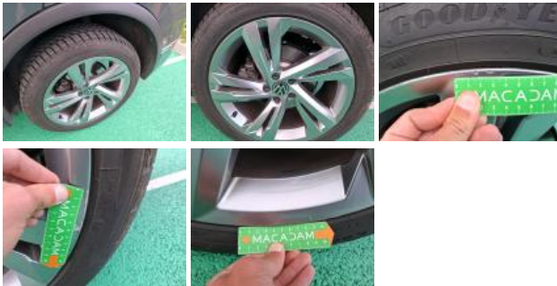
Tyre RR, Out of tolerance, Replace
