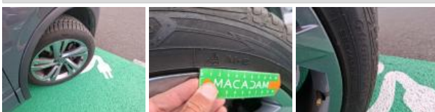
Tyre FR, Out of tolerance, Replace
