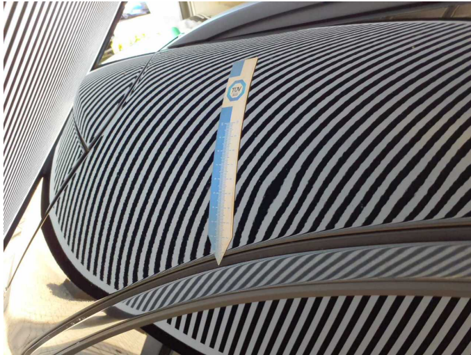
Damage 6: Roof: Roof rail - right side - Deformed - Repair and paint
