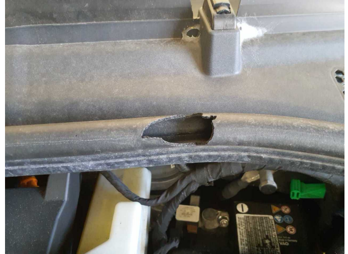
Damage 2: Engine: Engine cover (+ Dichtung) - Damage caused by marten / rodent - Replace
