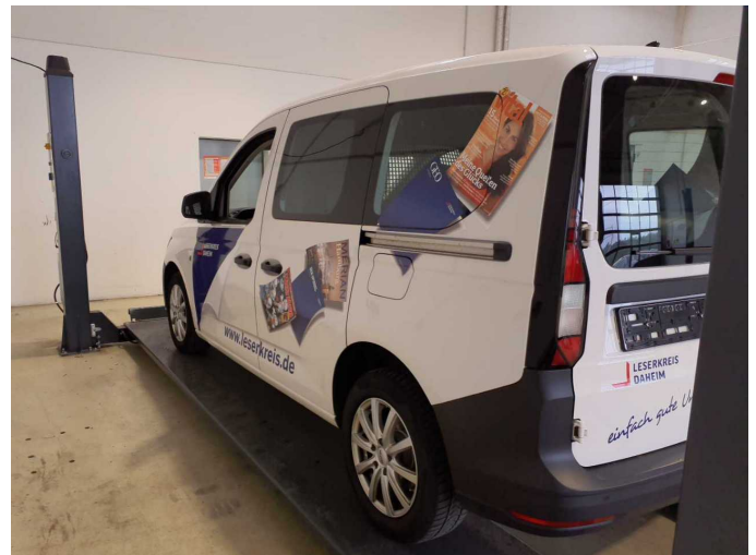
Damage 4: Body: Body - Glued / labelled - De-glove / neutralise
