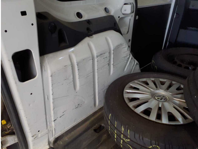
Damage 8: Body: Wheel well - rear left side - Deformed - Repair and paint
