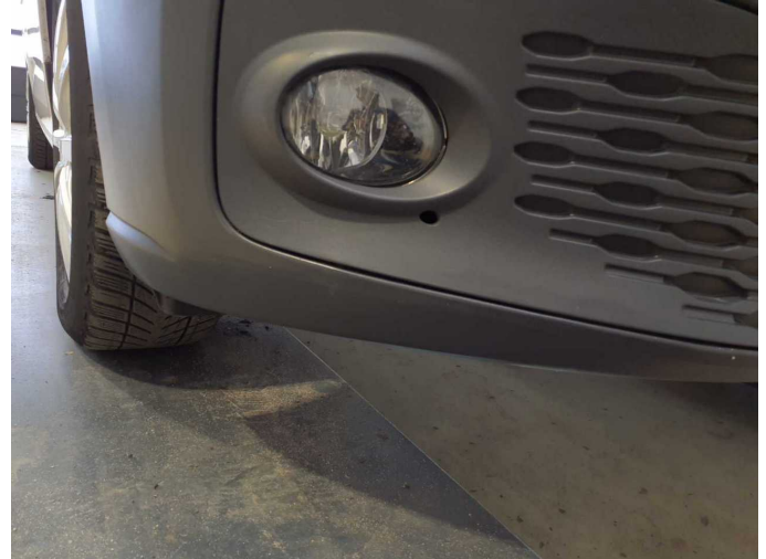
Damage 7: Front bumper: Front bumper - Scratched - Replace
