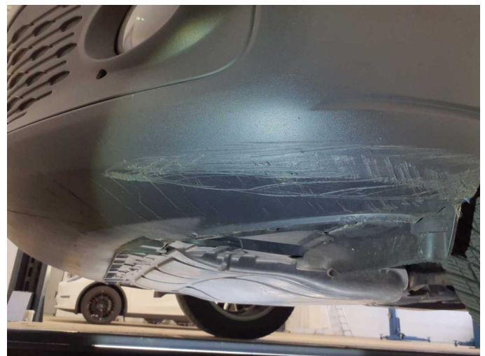
Damage 7: Front bumper: Front bumper - Scratched - Replace
