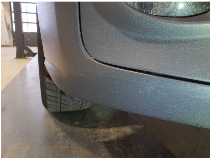
Damage 7: Front bumper: Front bumper - Scratched - Replace
