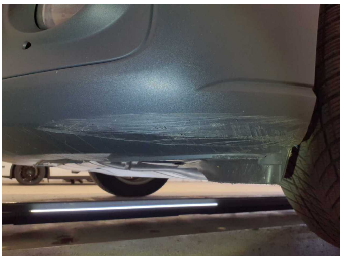
Damage 7: Front bumper: Front bumper - Scratched - Replace
