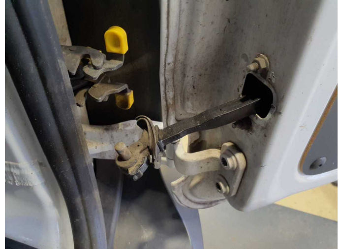
Damage 2: Boot lid / rear door: Door check strap / arrestor - Damaged - Replace
