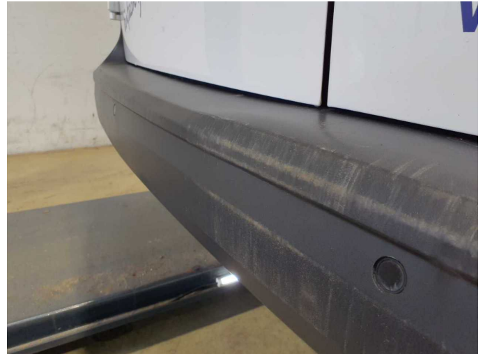
Damage 6: Rear bumper: Rear bumper - Deformed - Replace
