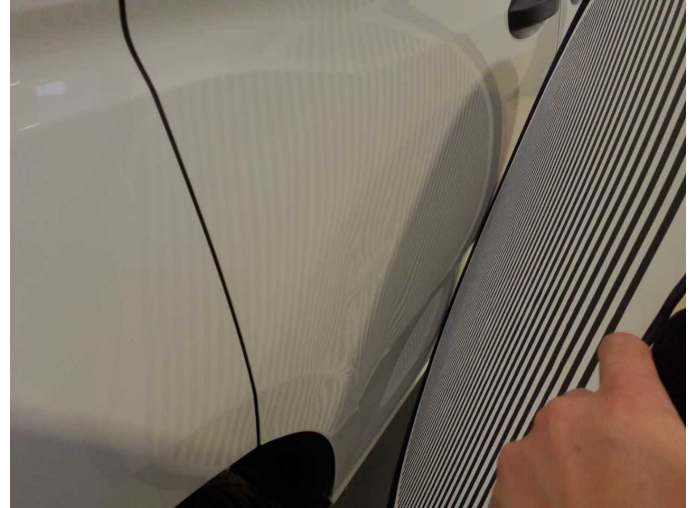
Damage 10: Sliding door, right: Sliding door with glass panel - Deformed - Repair and paint
