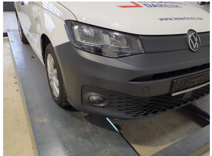
Damage 7: Front bumper: Front bumper - Scratched - Replace
