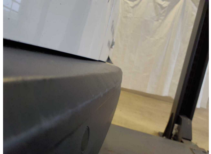
Damage 6: Rear bumper: Rear bumper - Deformed - Replace
