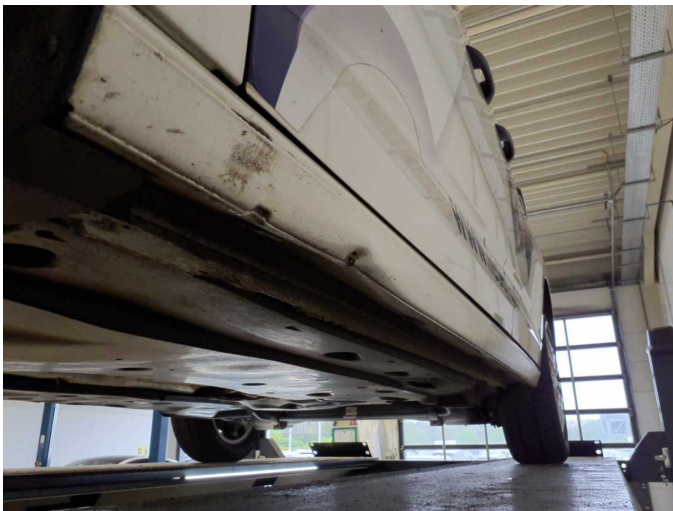
Damage 9: Sill - left side: Sill - Deformed - Repair and paint
