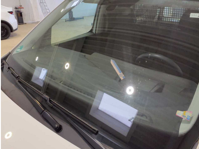
Damage 11: Vehicle glazing: Windscreen with lane departure assistant - Stone chips - Replace
