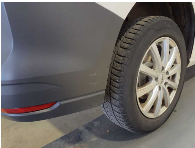
Damage 6: Rear bumper: Rear bumper - Deformed - Replace
