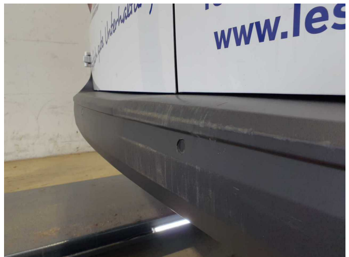
Damage 6: Rear bumper: Rear bumper - Deformed - Replace
