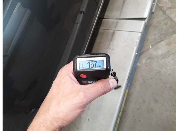
Repainting 1: Door - rear right side, Door - front left side, Door - front right side
