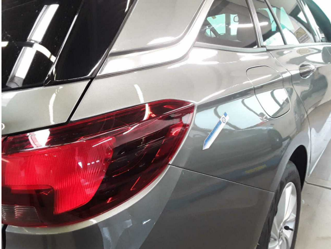
Damage 1: Side panel - rear right side: Side panel (Schleifspuren) - Unprofessionally repaired - Smart repair
