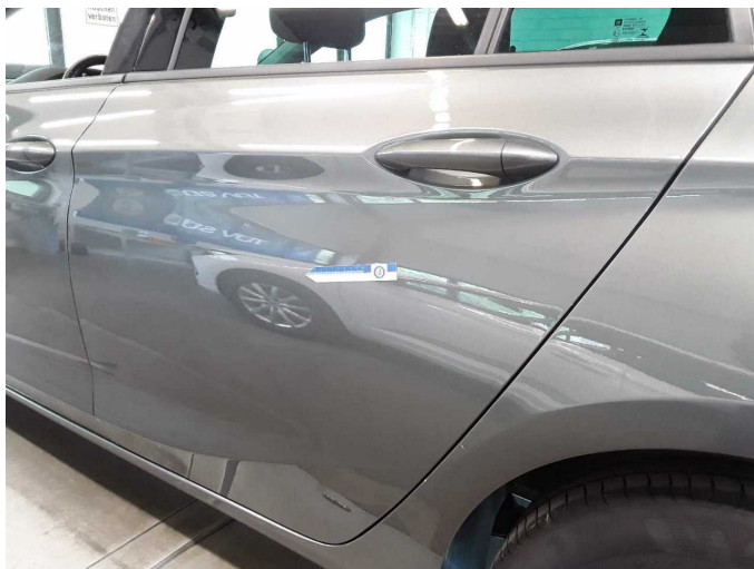
Damage 10: Door - rear left side: Door - Dent / paintcoat damage - Repair and paint
