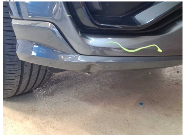
Damage #5: Front bumper: Front bumper - Deformed - Replace
