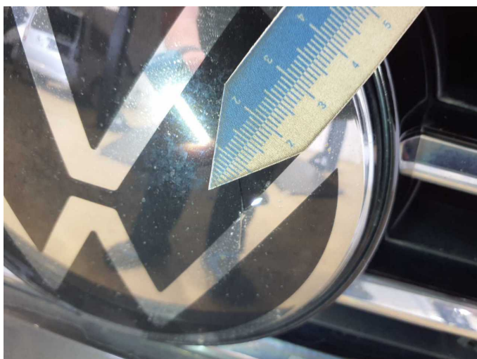
Damage 7: Front structure: Emblem - Broken / torn - Replace
