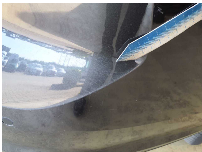
Damage 11: Rear bumper: Rear bumper - Scratch(es) - Paint
