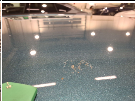
Roof / - / Paint etching
