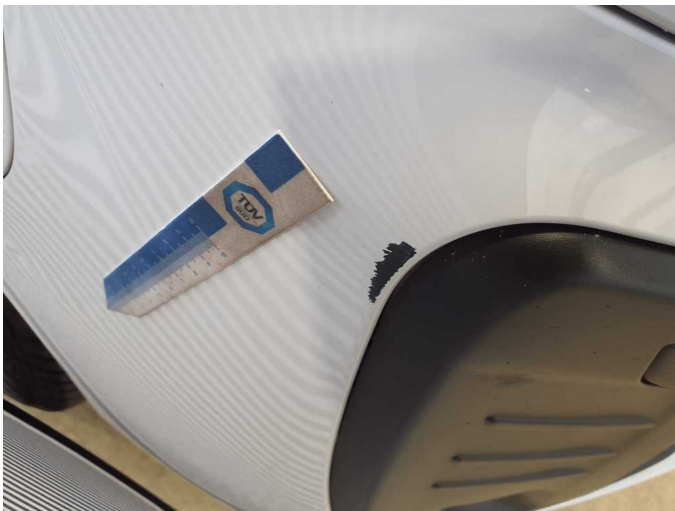
Damage 9: Front bumper: Front bumper - Dent / paintcoat damage - Paint
