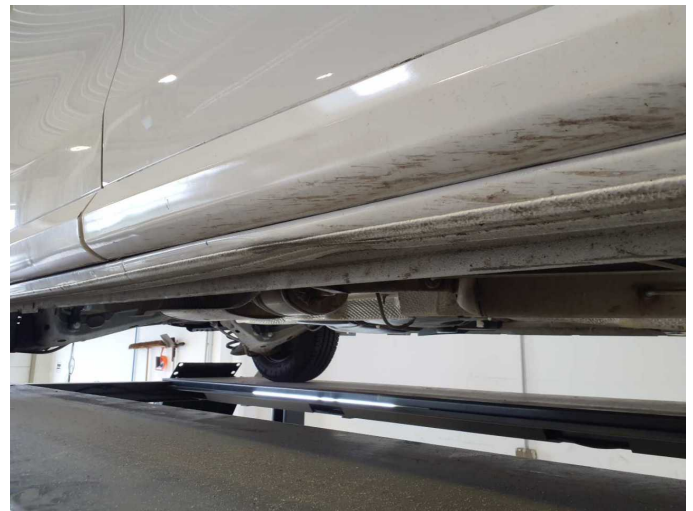
Damage 8: Sill - right side: Sill - Deformed - Repair and paint
