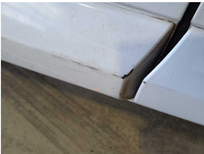
Damage 2: Door - rear right side: Brightware - lower - Scratch(es) - Smart repair
