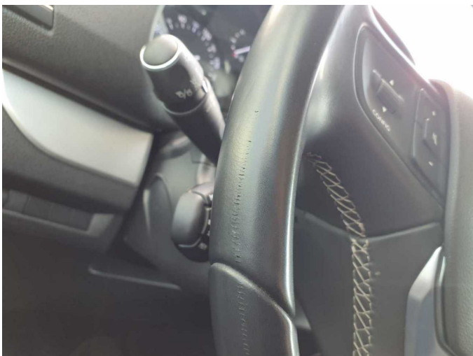
Damage 5: Steering system: Steering wheel - Scratch(es) - Smart repair
