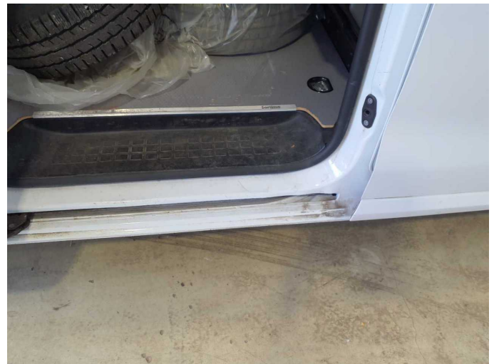
Damage 10: Side panel - rear right side: Sill - Dent / paintcoat damage - Repair and paint
