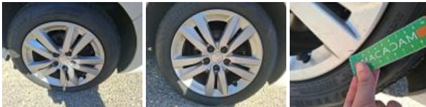
Tyre RR, Out of tolerance, Replace
