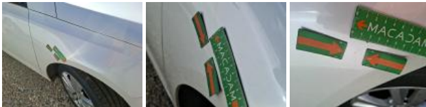
Door RR, Dent(s), Repair and paint (complete)
