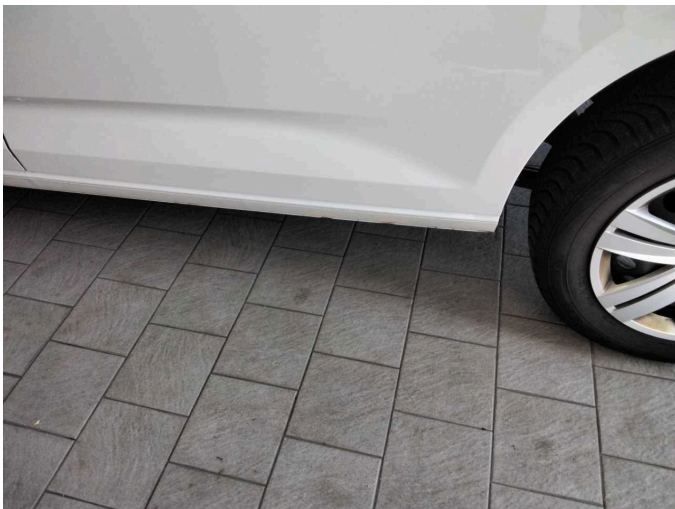
Damage 4: Sill - left side: Sill - Dent / paintcoat damage - Repair and paint
