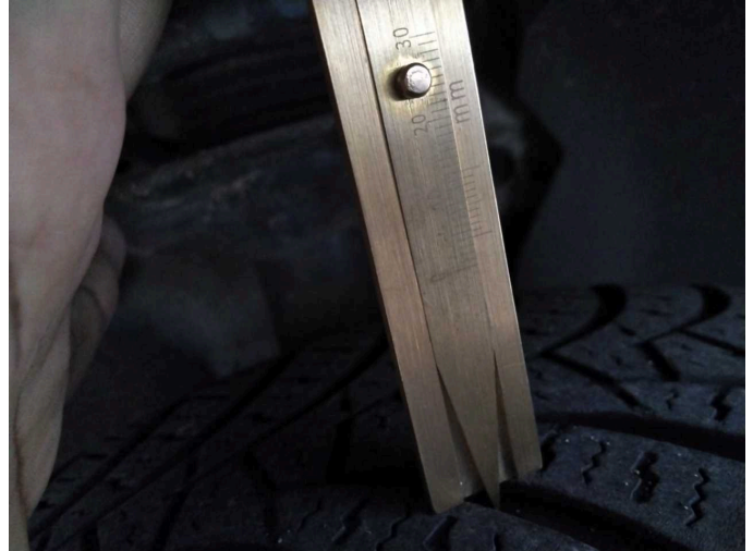
Damage 3: Wheel / tyres: Wheelset - complete (3mm) - does not meet manufacturer specifications - Replace
