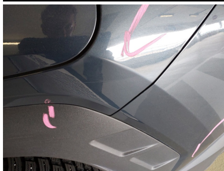
Kotflügel / Hinten Links / Delle
