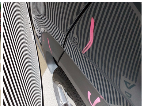
Kotflügel / Hinten Links / Delle
