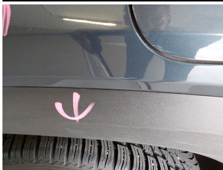
Kotflügel / Hinten Links / Delle
