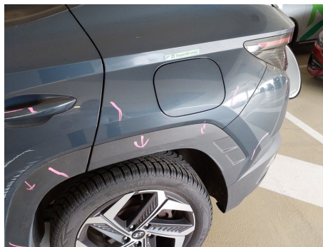
Kotflügel / Hinten Links / Delle
