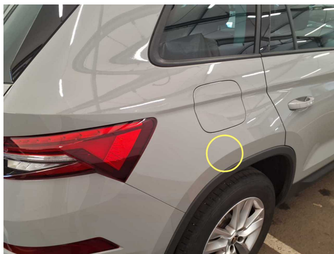
Damage 2: Side panel - rear right side: Side panel - Dent / paintcoat damage - Repair and paint
