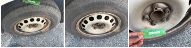
Wheel cover RR, Missing, Replace
