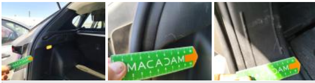
Rubber seal for boot lid, Tear, Replace
