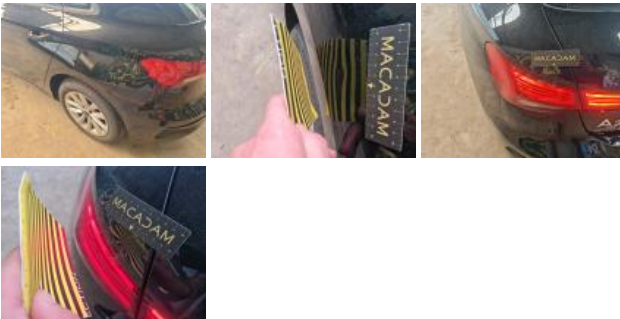
Rear light L, Broken, Replace
