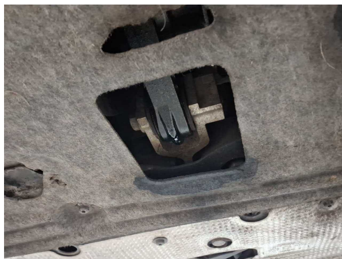
Damage 5: Engine: Engine - Leaking - Perform diagnosis
