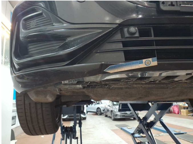
Damage 7: Front bumper: Front bumper - Scratch(es) - Paint
