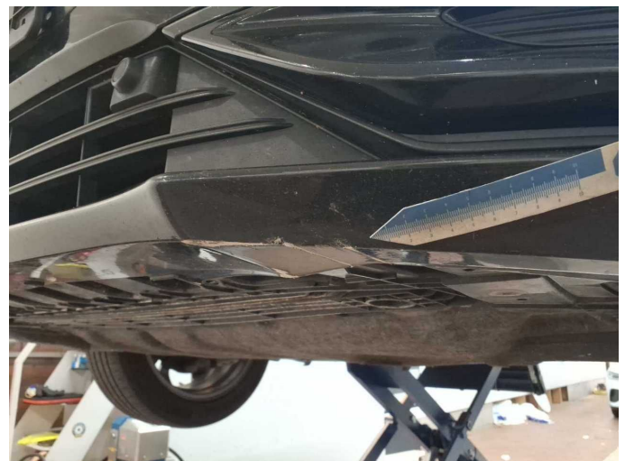
Damage 7: Front bumper: Front bumper - Scratch(es) - Paint
