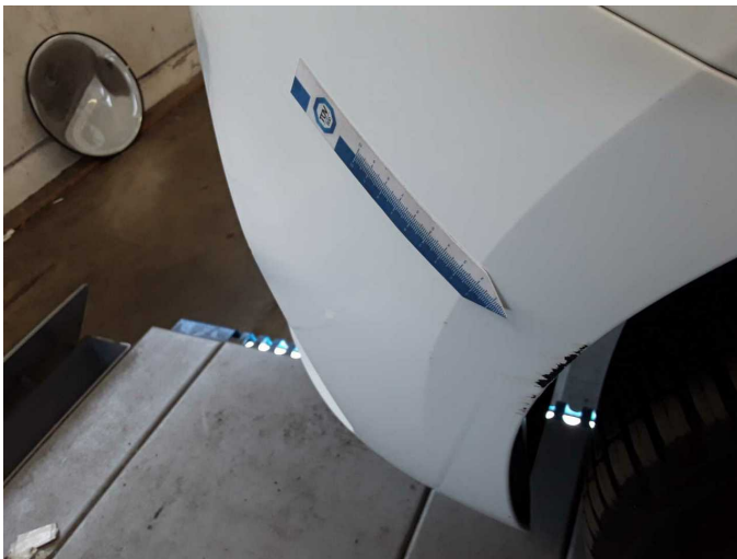
Damage 3: Front bumper: Front bumper - Scratched - Paint
