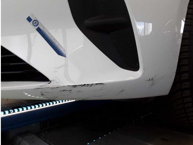
Damage 3: Front bumper: Front bumper - Scratched - Paint
