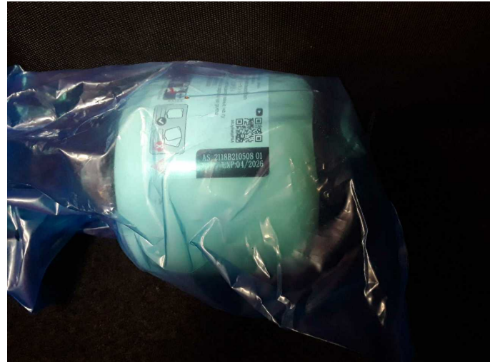
Damage 1: Equipment: Tirefit filler - Expired - Replace
