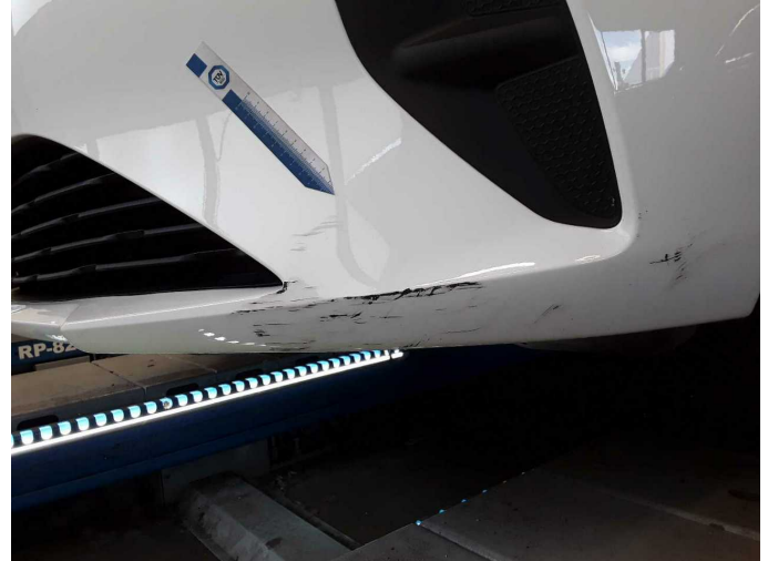
Damage 3: Front bumper: Front bumper - Scratched - Paint
