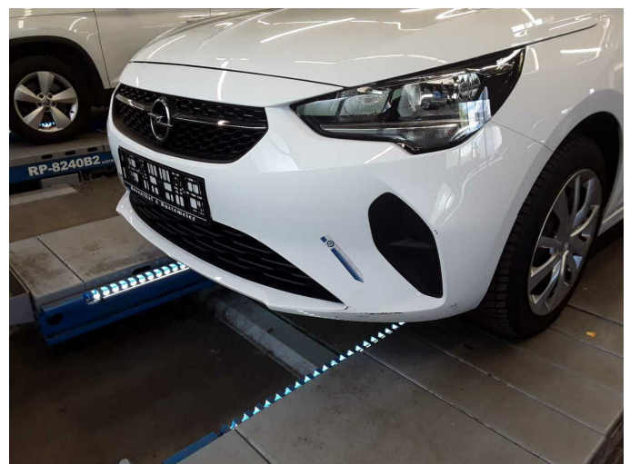
Damage 3: Front bumper: Front bumper - Scratched - Paint
