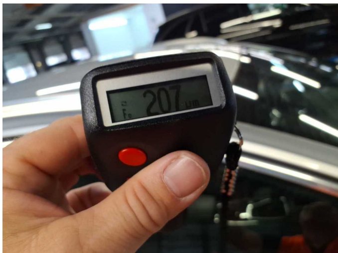
Repainting 2: Roof rail - right side
