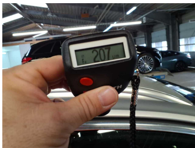
Repainting 2: Roof rail - right side
