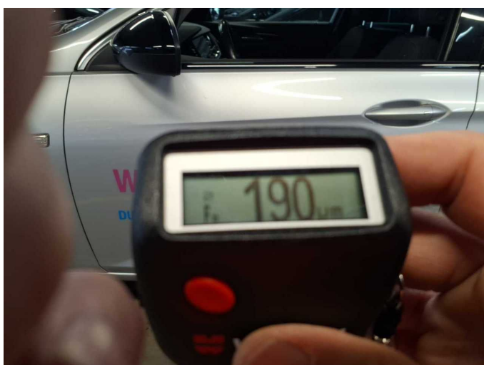
Repainting 9: Door - front left side
