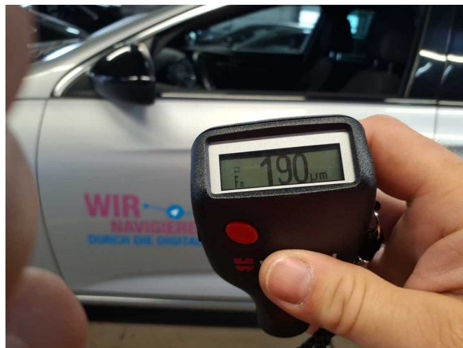
Repainting 9: Door - front left side
