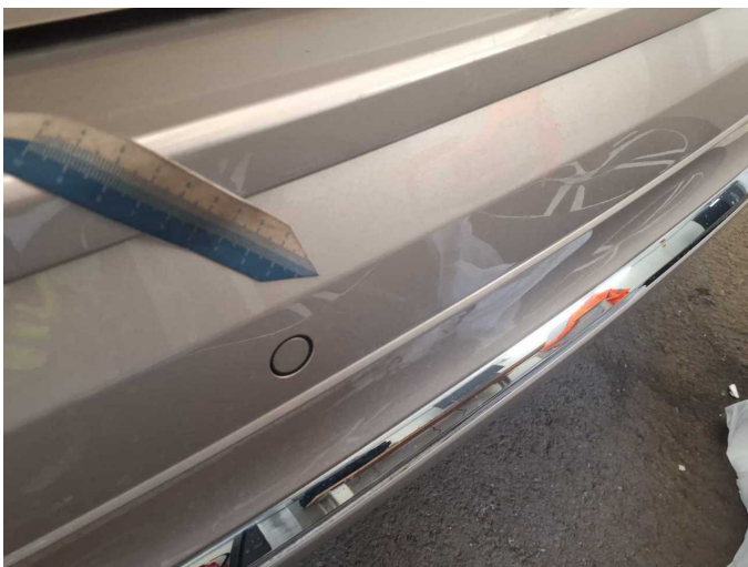
Damage 8: Rear bumper: Rear bumper - Scratch(es) - Paint
