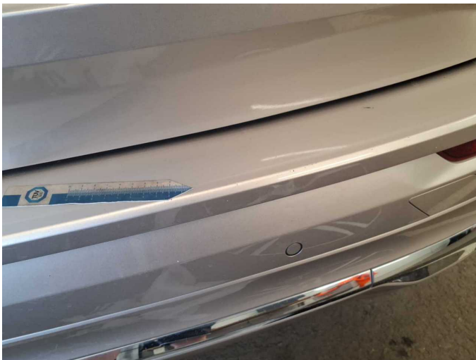
Damage 8: Rear bumper: Rear bumper - Scratch(es) - Paint
