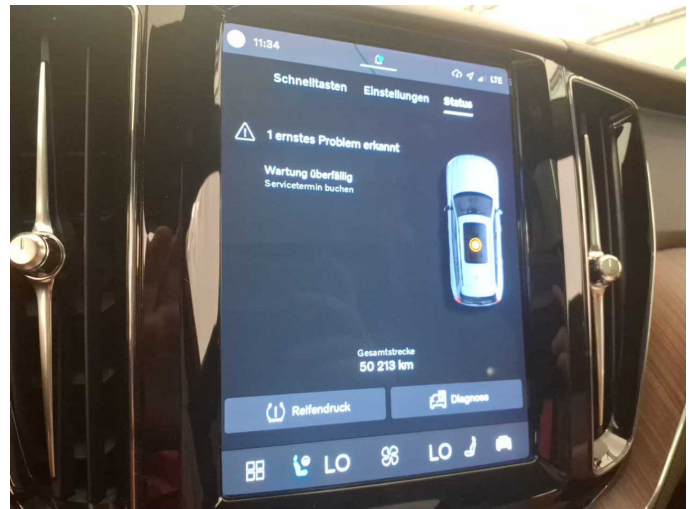
Damage 6: Misc.: Inspection / maintenance - Expired - Perform
