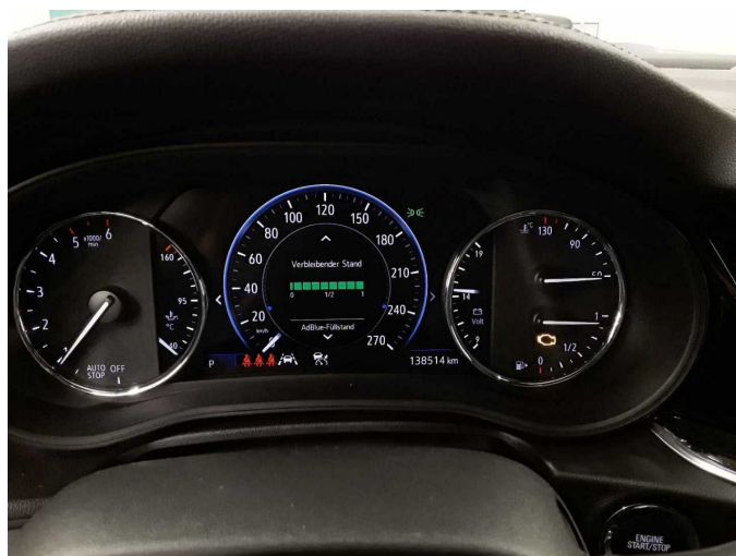
Damage 4: Instrument panel: Indicator light (Motorkontrolle) - on - Perform diagnosis
