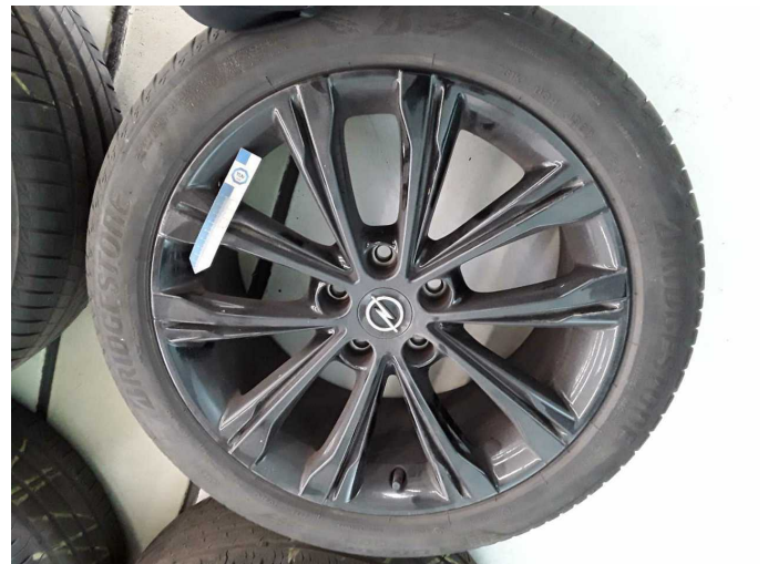
Damage 6: 2nd wheel set: 1 alloy rim (Wurde bearbeitet) - Unprofessionally repaired - Replace
