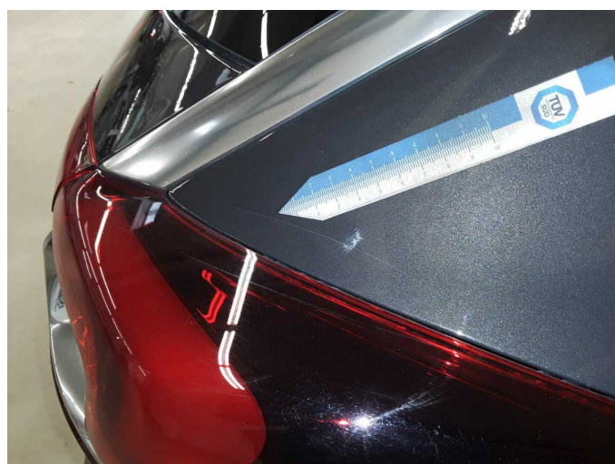
Damage 8: Side panel - rear right side: Side panel - Scratch(es) - Repair and paint
