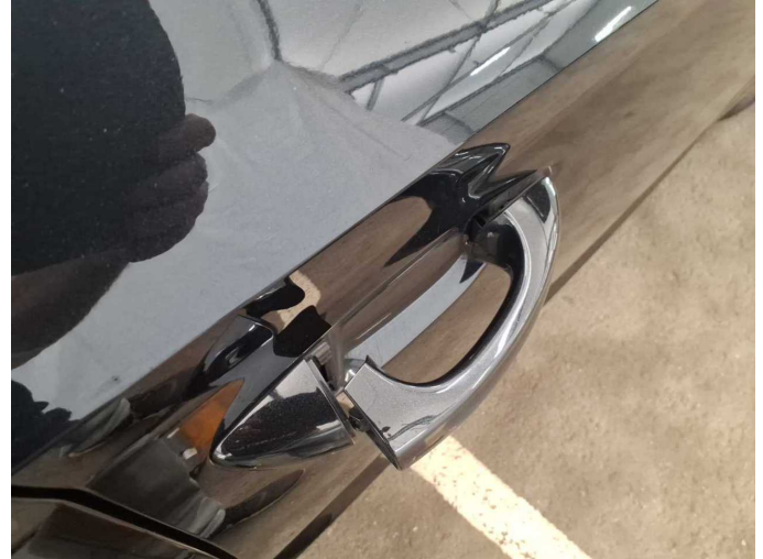
Damage 1: Door - front right side: Door handle - outside (Harkt/Klemmt fest) - Sub-function - Replace
