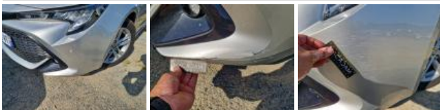
Bumper moulding FL, Broken, Replace and paint
