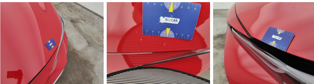
Front Bonnet // Repair & Painting-scratch + dent
