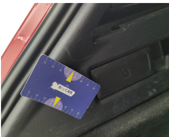
Trunk Compartment / Side Cover Left / Replace-scratch
