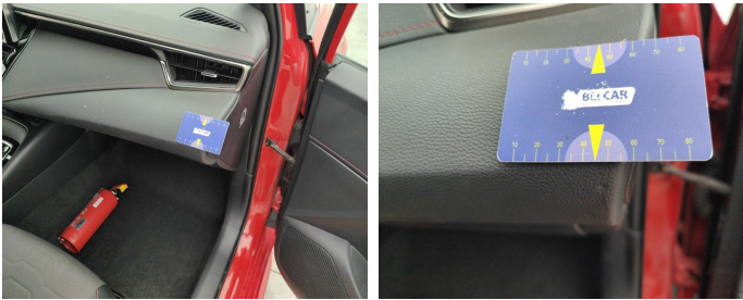
Dashboard // Replace Completely-scratch
