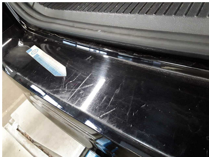
Damage 2: Rear bumper: Rear bumper - Scratched - Paint
