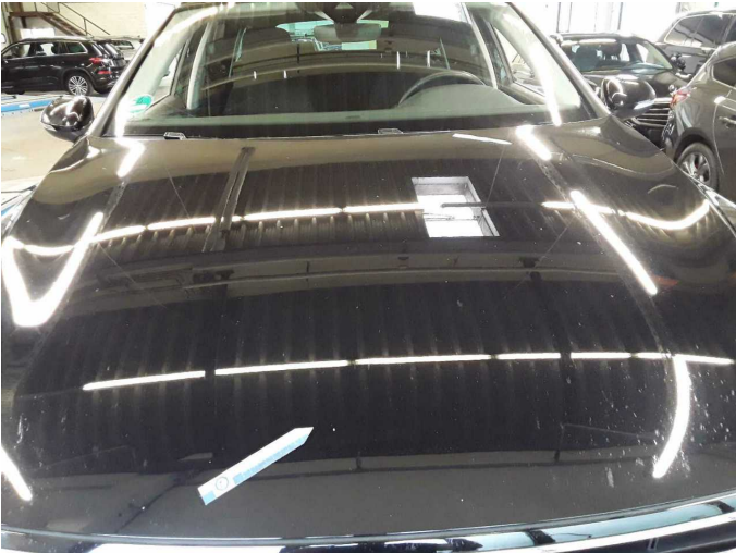
Damage 1: Bonnet: Bonnet - Dent / paintcoat damage - Repair and paint
