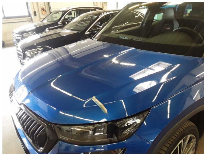
Wear and tear 3: Bonnet: Bonnet - Dent / paintcoat damage - Smart repair
