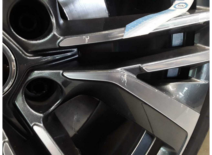
Wear and tear 1: Wheel / tyres: Alloy rim - front left side (Eingelaufen) - No deduction
