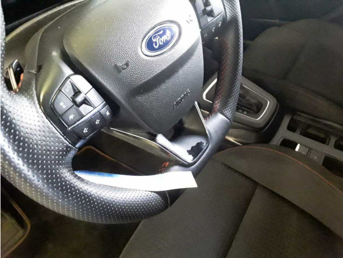
Damage 3: Steering system: Steering wheel - Worn - Loss in value
