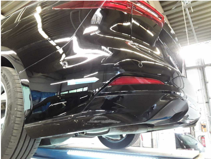
Damage 5: Rear bumper: Rear bumper - Scratch(es) - Paint
