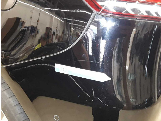
Damage 11: Rear bumper: Rear bumper - Scratch(es) - Paint
