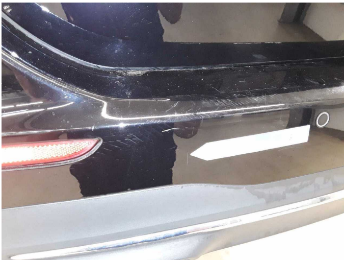
Damage 11: Rear bumper: Rear bumper - Scratch(es) - Paint
