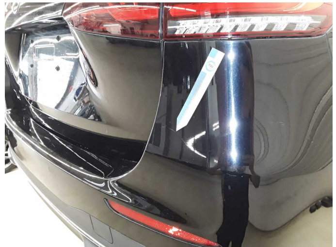
Damage 11: Rear bumper: Rear bumper - Scratch(es) - Paint
