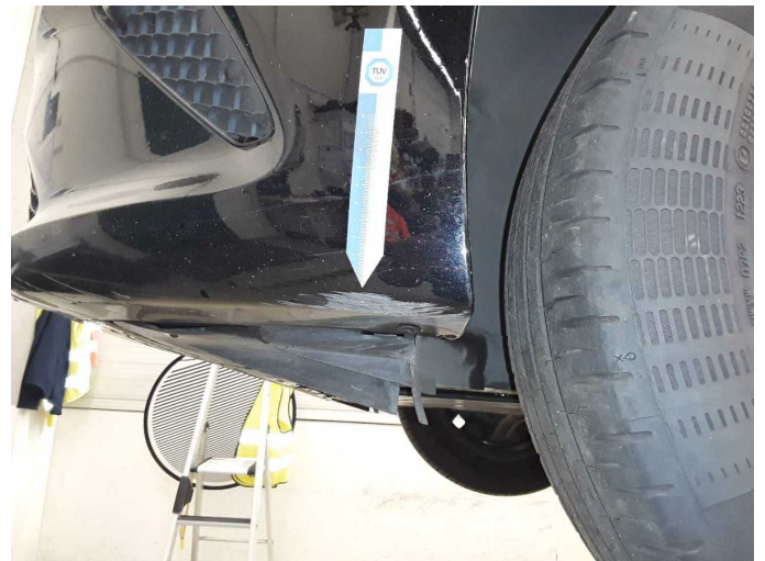
Damage 10: Front bumper: Front bumper - Scratch(es) - Paint
