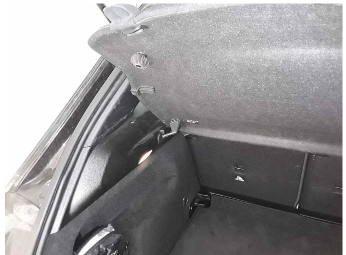
Damage 7: Interior: Rear shelf - Broken / torn - Replace
