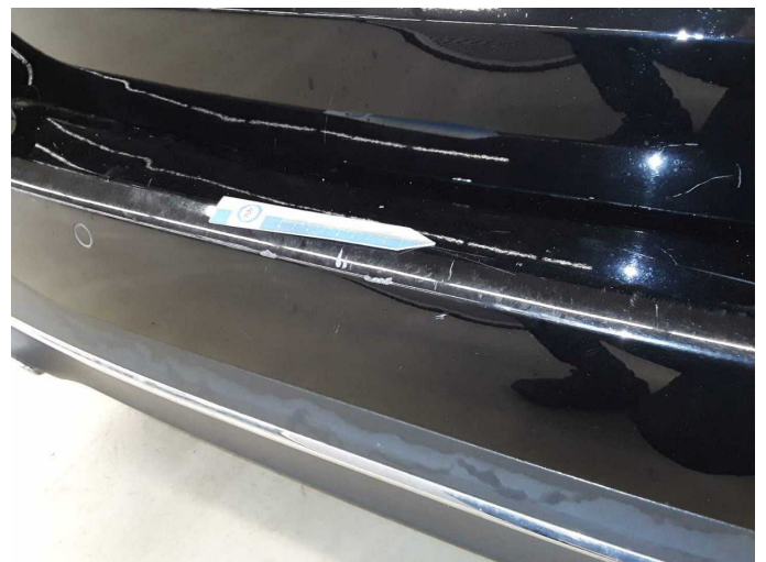
Damage 11: Rear bumper: Rear bumper - Scratch(es) - Paint
