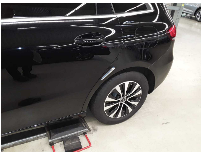
Damage 9: Side panel - rear left side: Side panel - dent(s) - Smart repair
