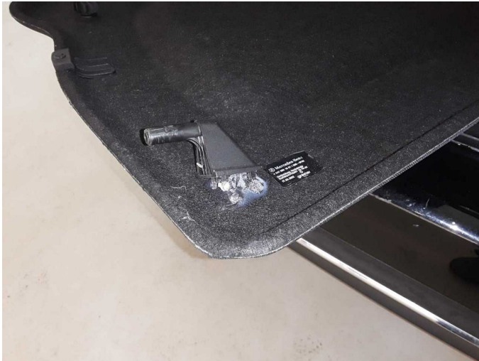
Damage 7: Interior: Rear shelf - Broken / torn - Replace
