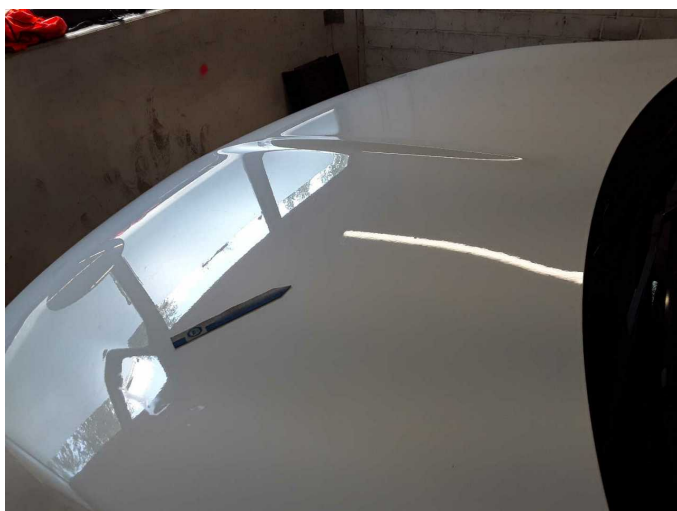
Damage 2: Bonnet: Bonnet (3;dellen) - dent(s) - Smooth repair work
