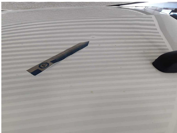
Damage 5: Roof: Roof - dent(s) - Smooth repair work
