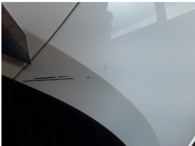
Damage 7: Front bumper: Front bumper - Scratch(es) - Paint
