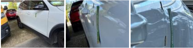
Door RR, Dent(s), Repair and paint (complete)
