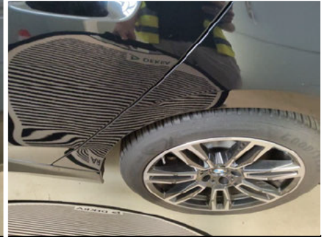
Kotflügel / Hinten Links / Delle
