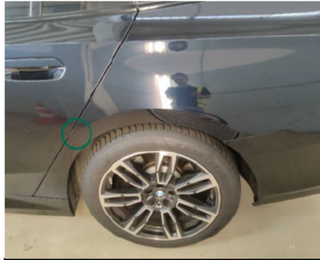
Kotflügel / Hinten Links / Delle
