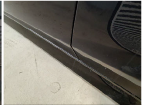
Tür / Vorne Links / Kratzer
