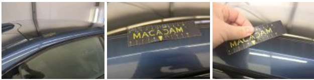
Boot lid covering R, Scratch(es), Replace
