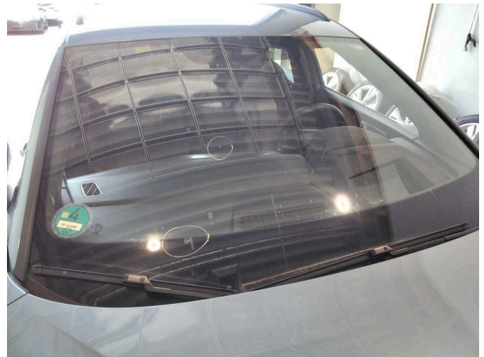
Damage 6: Vehicle glazing: Windscreen - Stone chips - Replace
