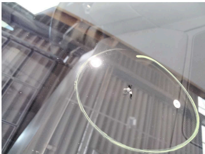
Damage 6: Vehicle glazing: Windscreen - Stone chips - Replace
