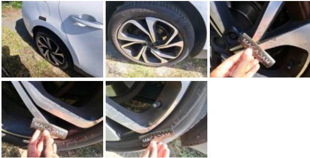
Tyre FR, Out of tolerance, Replace
