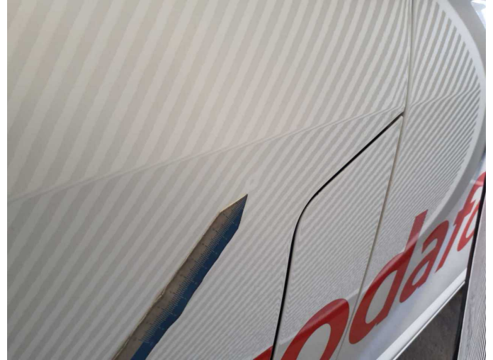
Damage 2: Door - front left side: Door - dent(s) - Smart repair
