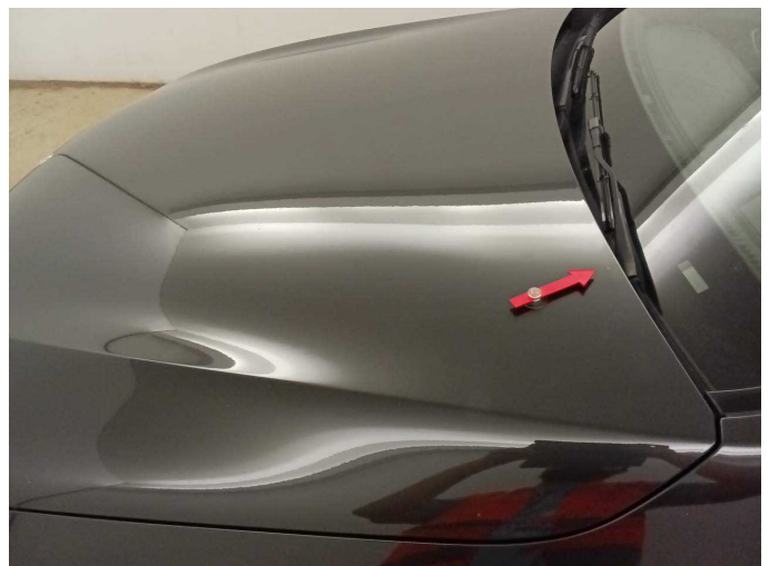
Damage 6: Bonnet: Bonnet - Stone chips - Paint
