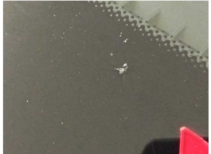
Damage 7: Vehicle glazing: Windscreen - Stone chips - Replace
