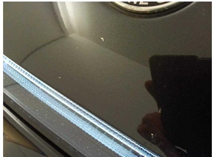
Damage 6: Bonnet: Bonnet - Stone chips - Paint
