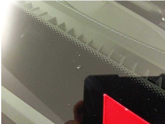
Damage 7: Vehicle glazing: Windscreen - Stone chips - Replace
