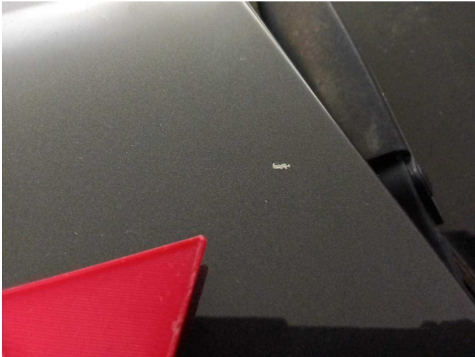
Damage 6: Bonnet: Bonnet - Stone chips - Paint
