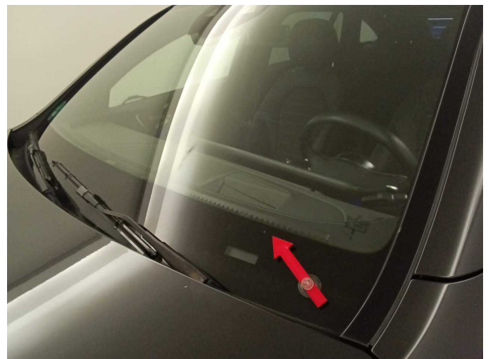
Damage 7: Vehicle glazing: Windscreen - Stone chips - Replace
