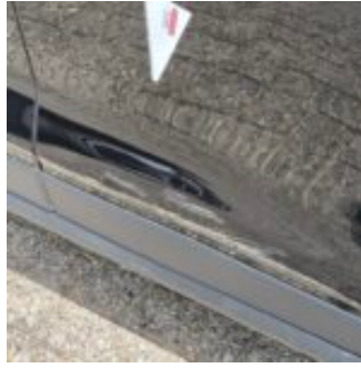
Damage Type Dent(s) & Scratch(es)
