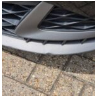
Damage Type Small dent(s)
