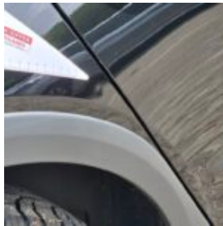
Damage Type Small dent(s)
