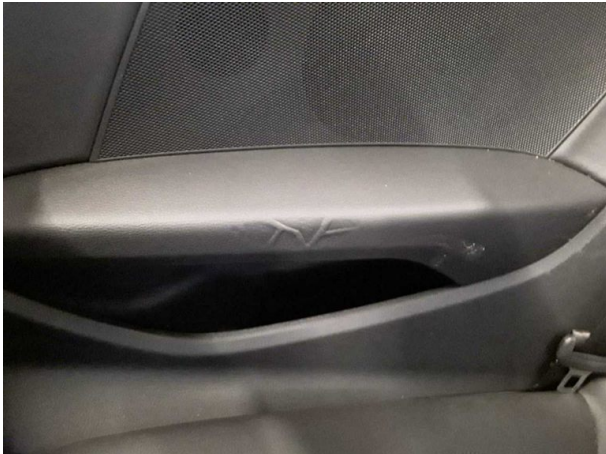
Damage #2: Interior: Interior (Druckstellen) - No deduction
