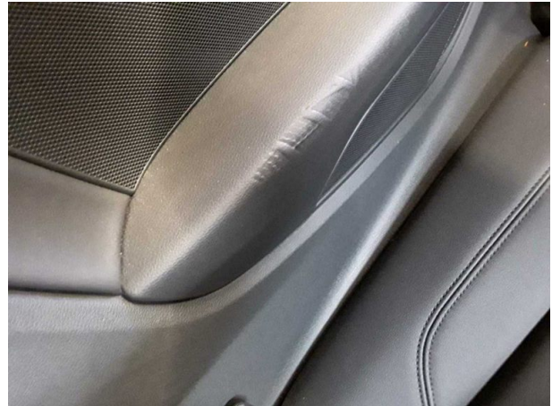
Damage #2: Interior: Interior (Druckstellen) - No deduction
