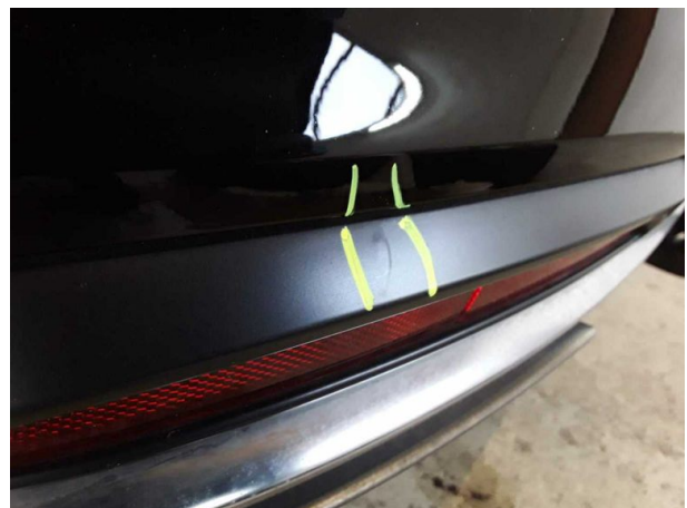
Damage #5: Rear bumper: Spoiler (Druckstellen) - Loss in value
