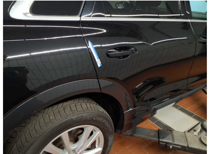
Damage 1: Door - rear right side: Door edge - Scratch(es) - Smart repair
