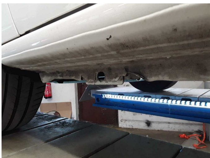
Damage 2: Sill - left side: Sill - Deformed - Repair and paint
