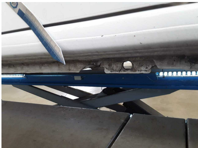
Damage 3: Sill - right side: Sill - Deformed - Repair and paint
