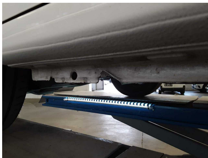
Damage 3: Sill - right side: Sill - Deformed - Repair and paint
