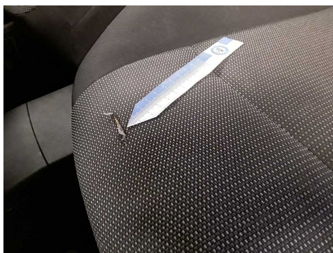
Damage 4: Seat - front: Seat cover - left side - Porous / cracked - Replace
