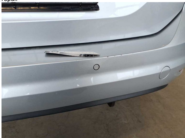
Damage #2: Rear bumper: Rear bumper - Scratch(es) - Repair and paint
