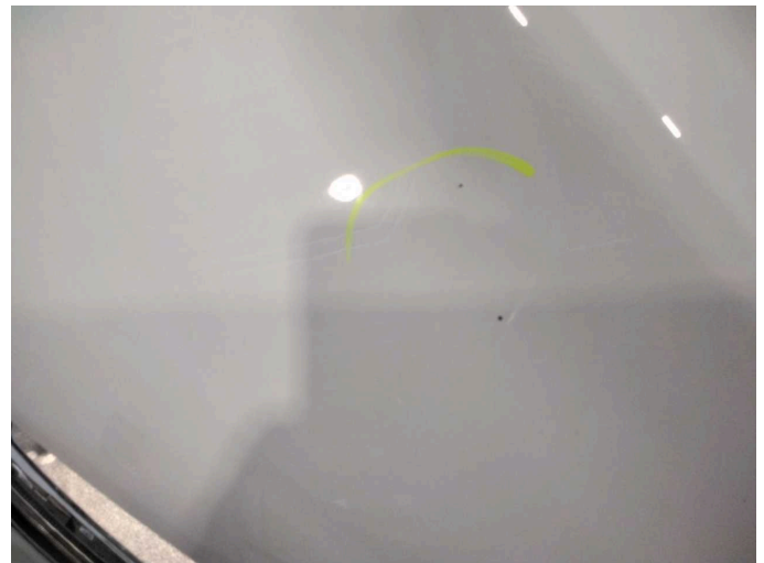
Damage 7: Bonnet: Bonnet - Stone chips - Paint
