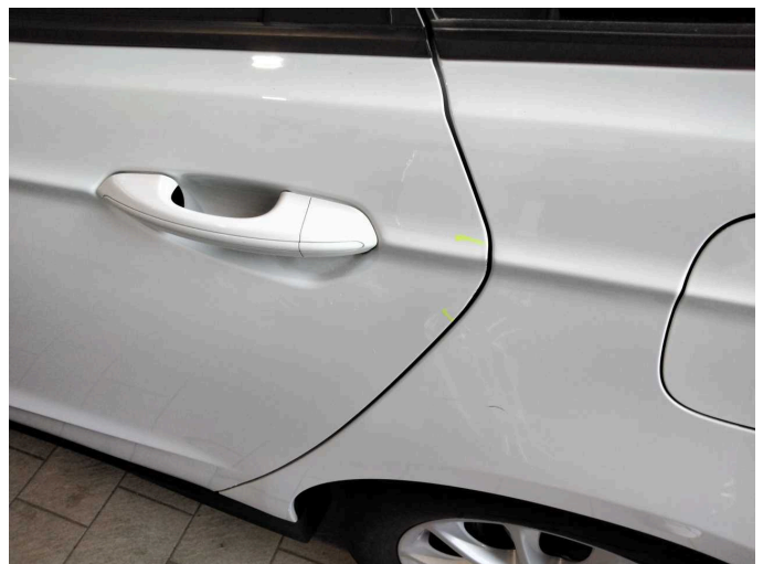
Damage 2: Door - rear left side: Door edge - Scratch(es) - Smart repair
