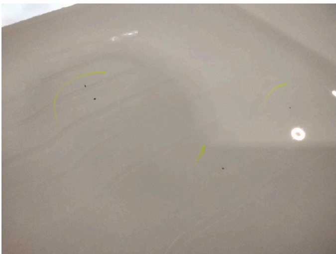
Damage 7: Bonnet: Bonnet - Stone chips - Paint
