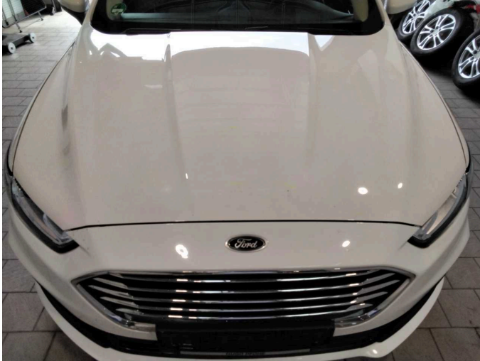
Damage 7: Bonnet: Bonnet - Stone chips - Paint
