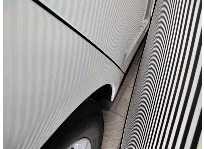
Wear and tear 2: Side panel - rear right side: Side panel - dent(s) - No deduction
